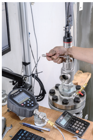
申錫自社開発- 安全弁排出性能試験台 Hopeet In-house Developed Safety Valve Discharge Performance Testing Bench
