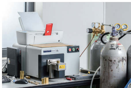
卓上型固体発光分光分析装置 HITACHI FOUNDRY-MASTER Material Analyzer Spectrometer
