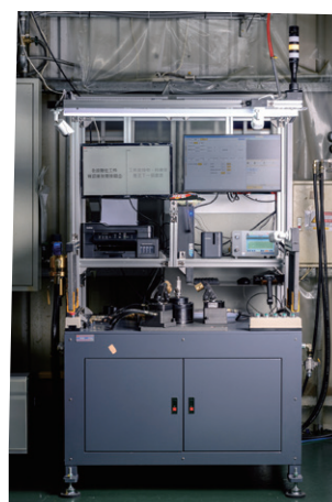
申錫自社開発- 一体型圧力・漏れ試験台 Hopeet In-house Developed Pressure Testing & Leak Detection Bench
