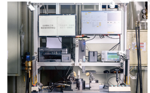
申錫自研-一站式測壓檢漏平台 Hopeet In-house Developed Pressure Testing & Leak Detection Platform
