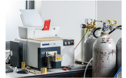
材質分析分光儀 HITACHI FOUNDRY-MASTER Material Analyzer Spectrometer
