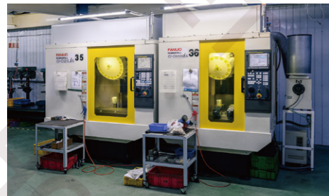
FANUC ROBODRILL *2 銑床 FANUC ROBODRILL milling machine
